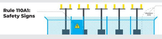
Figure 110-1: Safety Clearance to Electric Supply Station Fences.
